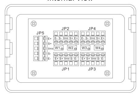
JP1~JP4 for load cell input,JP5 for summed signal output. W1~W4 for signal trimming,corresponding to JP1~JP4 respectively.
